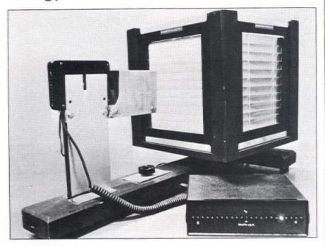
Microscanning unit which reads heat transfer of venetian blind slats is demonstrated by Hunter Douglas Inc. Unit utilizes a light bulb which radiates both light and heat equally to an assembly of venetian blind slats mounted on a rotating quadrangle. Fixed position sensing instrument (microscanner) is
