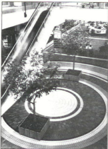
Buchtal Architectural Ceramics —A total of 65,000 sq. ft. of the firm's 4- by 8-in. unglazed tile was specified for Pittsburgh Allegheny Mall. Used in a three-color combination, these tiles provided abrasion-resistant paving that could be installed without closing the mall. Circle No. 239.
