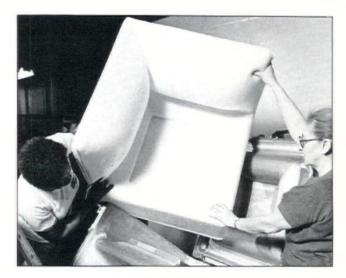
NEW MOLD ENABLES SOFA DESIGN BREAKTHROUGH Workers remove a new, modular, foam sofa from a specially designed mold at **Goodyear's** plant in Luckey, Ohio. Upholstered by Steelcase, sofa features a tubular steel frame. **Circle No. 254.**
