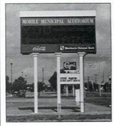
Venus 4000 electronic message/ animation center is an advanced microprocessor-based system that combines graphics, animation, and word messages. Displays are custom-designed to produce the correct message for individual users. Manufactured by Daktronics Inc., systems, such as Mobile Municipal Auditorium display (shown), feature large lampbanks that are controlled by Venus 4000. Circle No. 397.
