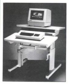
The Professional Marketing Group Inc. developed the "UFO 2000," an ergonomic workstation that permits control from a seated position. Front keyboard surface tilts five degrees and has a 10-inch vertical range. Rear surface tilts 15 degrees forward and back, and has a 10-inch vertical adjustment that accommodates any light/line-ofvision combination. Firm will match major panel manufacturers' colors and finish materials. Circle No. 254.
