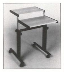
Facit offers a new terminal table which adjusts for operation from either seated or standing positions. Separate surfaces are provided for detached keyboard and screen terminals. Work space is expanded by adding side surfaces to left or right of keyboard or screen supports. To accommodate user's depth of vision, front surface can be moved forward or backward. Height adjustment ranges from 26- to 40-in. high. Graduated scales are affixed to both surfaces and serve as an adjustment guide.
