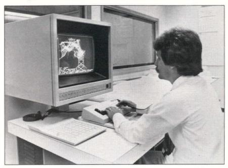
A computer-aided design and drafting center in Detroit was recently established by Efficient Engineering Co., an engineering service bureau headquartered in that city. Access to a full range of automated design, engineering, and drafting capabilities will be possible on a project basis or CADM rental. Using an Applicon 895 system with four-color stations, the facility will address a vari-
