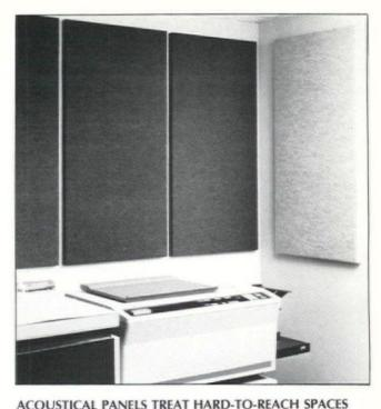
**Conved** expands its acoustical product line with Silent Accents sound absorbers. Designed for hard-to-reach spaces, panels measure 2-by 4-ft. or 2- by 6-ft. and feature an NRC rating of .90 to 1.00. Adhesive-backed strips enable no-tool installation. **Circle No. 390.**
