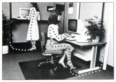
CleatStat mat from Rubbermaid instantly drains static electricity charges to a ground through the mat's ground cord. A one-megohm resistor built into the ground cord protects computer operators from accidental shock due to external electrical faults. Cleats hold mat in place on carpet. Varied shapes and sizes are available. **Circle No. 223.**
