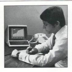
One-button information system eases access to assembly instructions, inventory data, and shipping requirements in industrial environments. Called Scanset, system is offered by Tymshare with automatic computer log-in, built-in modem, automatic phone dialer, and printer hook-up. Six multi-function programmable keys are monitored by the user or host computer. Up to 12 user-defined tasks can be assigned, enabling access to a range of frequently needed data bases. Circle No. 369.
