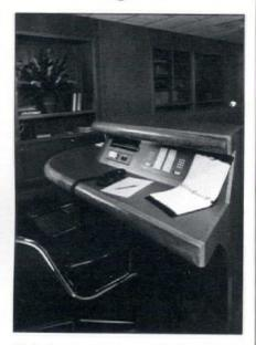
High-density telephone consoles from V Band Systems are specifically designed for traders working in brokerage firms and banks. Named the VK Family, consoles are offered in 30- to 120-line sizes with single or dual handsets. Other features include non-locking line keys, standard 1A2 lamp functions (wink, flash, and steady), and signal key for intercoms. **Circle No. 345**.
