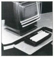
A totally adjustable CRT platform is also portable. Unit tilts, swivels, and slides for use on existing tables or desks housing video units. Mounting hardware is not required for use. Platform tilts 20 degrees up or down from horizontal position for glare reduction. Swivel capability of 360 degrees allows shared or angled operation. Unit slides up to 8 in. front-to-back to help reduce eye strain and adapt to individual preference. From Structural Concepts, unit is offered in various sizes.
