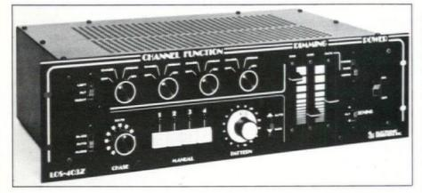
Electronic Designers Inc. has developed a four-channel light organ/chaser with 16-pattern microcontrol memory.
