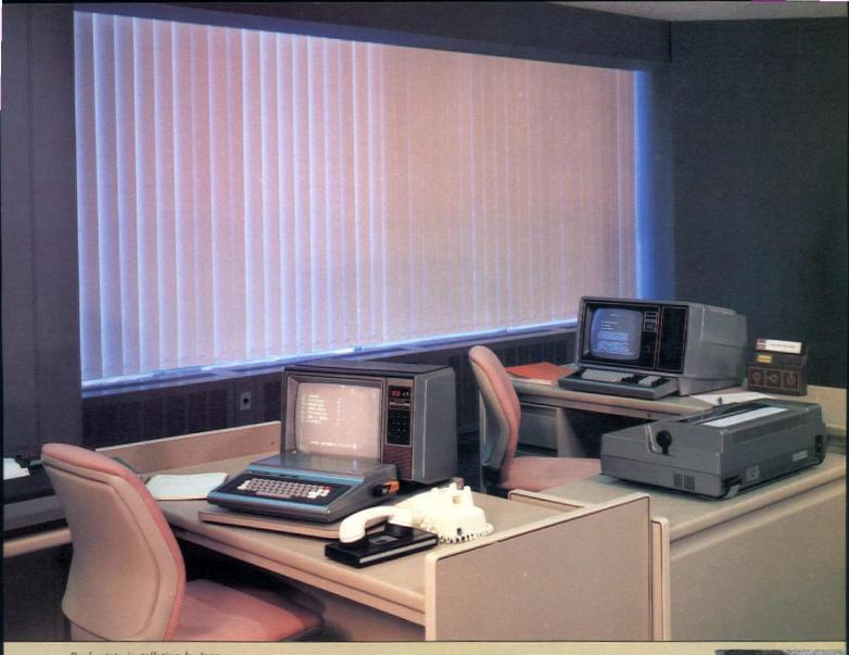
Real estate installation by Jane Victor (above) employs Radio Shack TRS-80 color computer with Extended Basic and 16K Memory, a realty software package, Model II Scripsit (word processing system), video screens, and Daisy Wheel printer-all on Steelcase workstations with Concentrx chairs.
