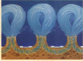
The urethane VORACEL backing penetrates the yarn tufts and locks them in. That produces a totally integrated carpet with high tuft lock and exceptional wearability.
