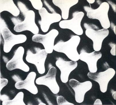
Micrographic blow-up of 300X, new Antron XL, 34 DPF (BCF) fourth generation nylon (left) shows total face fiber surface area of 19,500 cm<sup>2</sup>/oz, compared to 26,000 cm<sup>2</sup>/oz
