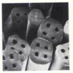
Magnification 250X of Antron<sup>®</sup> III nylon showing hollow filaments and round, anti-static filament.
