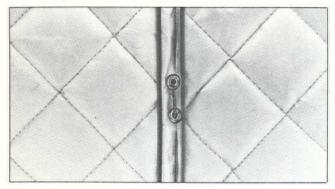
grey cloth facing, on one or two sides, is said to insure an easily cleaned, permanent outer shell impervious to oil, grease, and mildew. Class 1 rated building material can be mounted as a wall absorber, with an NRC rating of .70-.75, or hung as baffles to help control reverberations, or suspended as a semi-rigid curtain barrier to create an enclosure or divider, with sound reductions up to 21 dBA.
