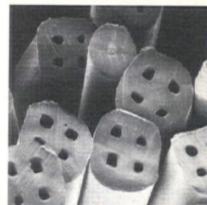
Magnification 250X of Antron® III nylon showing hollow filaments and round, anti-static filament.
