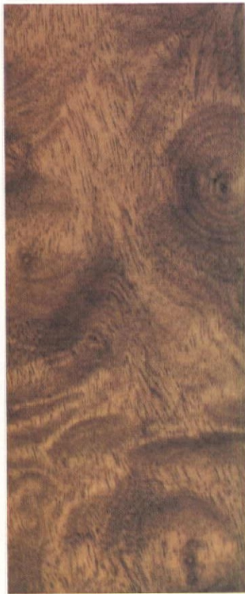
Camphor Burl comes from the Camphor tree in India. Note tight grain configuration, enlarged in scale.
