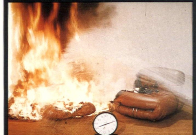
Time: 11 minutes. Standard chair, walls, floor (left) involved. Chair with VONAR 3 (right) is out.
