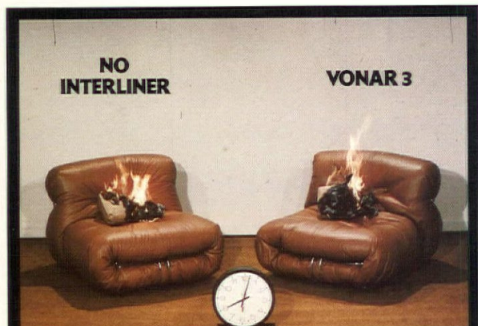
Time: 2 minutes into the test. Identical ignition sources nearly consumed.
