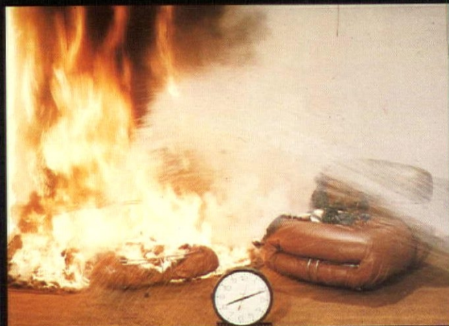
Time: 11 minutes. Standard chair, walls, floor (left) involved. Chair with VONAR 3 (right) is out. Chairs for this test provided by and available from Atelier International, Ltd.
