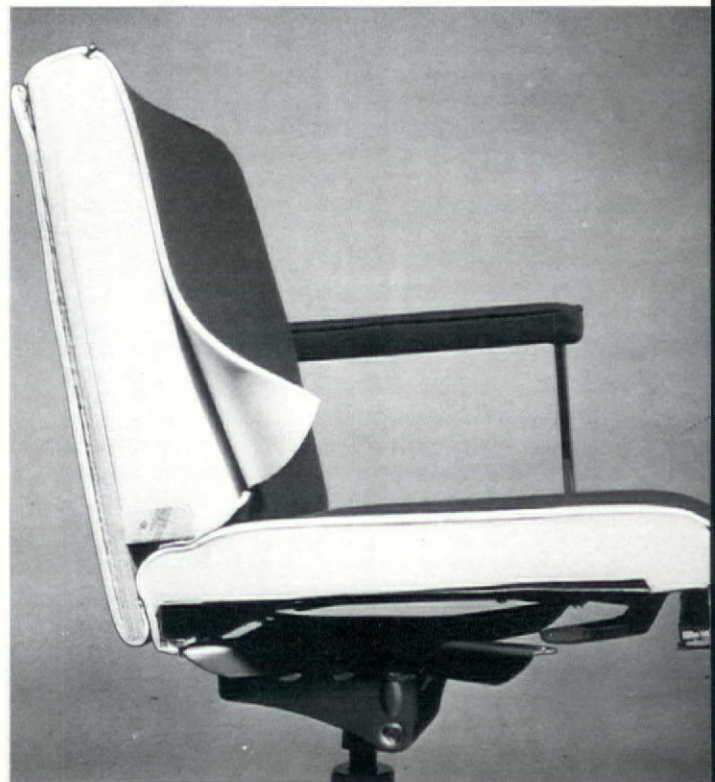
Cutaway of standard office chair shows "Vonar" interliner coated to undersurface of upholstery fabric. Other methods of installation include use of "Vonar" as separate layer applied between fabric and cushioning material and use of "Vonar" as an envelope over cushioning material. Time lapse photography shows four double sheets of newspaper being ignited on upholstered seats of standard office chairs, the one to the left constructed without "Vonar" interliner, the one to the right constructed with it. Newspaper is ignited at 2:00; flames on chair at left, flames charring fabric of chair at right at 2:04:30; almost total consumption by flames of chair at left, continuing flames but protection of cushioning of chair at right at 2:15.
