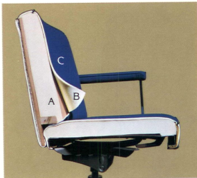
A. Standard polyurethane cushioning foam. B. A layer of VONAR 3 interliner coated on back of fabric. C. Standard nylon upholstery fabric.
