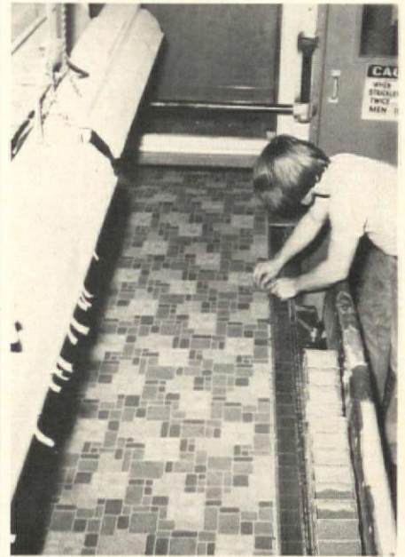
A line inspector corrects minor imperfections in part of the August 9 run of Armstrong's most popular style of embossed linoleum. This was the final run in the sixty-five-year history of Armstrong linoleum.
