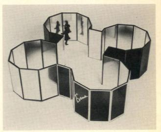
lighting hardware, the landscape system requires no architectural support and can be put in place overnight. Panels may be specified in clear or opaque finishes, are hinged to allow for unlimited combination and configuration.
