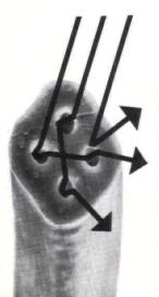
How "Antron" hides soil. Its filament structure is unique, as shown in this magnified (650×) cross section. The four precisely-placed hollow cores scatter light like the facets of a diamond to minimize the dulling effect of soil, while helping to retain color clarity and luster.
