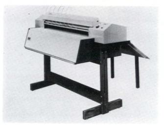
and copy material into the machine. Finished whiteprint and original are processed automatically. Since dry ammonia development is used, no liquid enters the machine, and no special plumbing or wiring is required.
