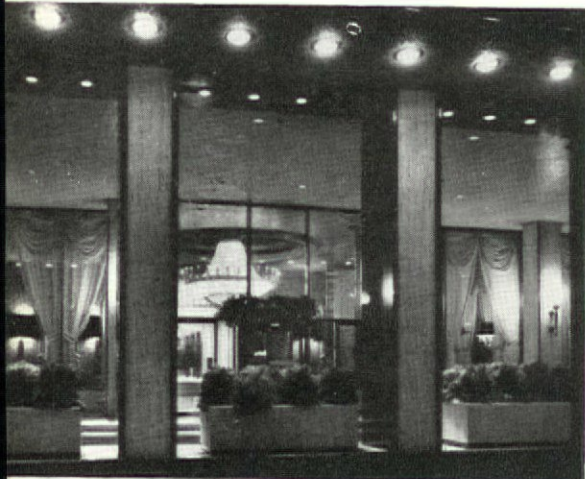
Lighting creates a lively, exciting ambience at Kennedy House apartment lobby. Visible from afar, a 12-foot diameter, 9-foot high chandelier glistens through glass walls and playfully casts its glow in an outdoor reflecting pool. Large bronze wall lanterns are placed on travertine columns, and the cement canopy over the drive has down spots to further light the way, while the entire lobby facade is flood-lighted with overhead lamps. Tom Lee Ltd., interior designer for the lobby, created all the lighting effects.
