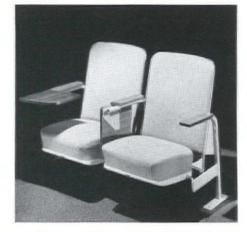
feature of Heywood-Wakefield's TC 477 FTA auditorium seating. Each chair is affixed to a single, heavy-duty tubular steel column, and supports adapt to level and sloping floors, as well as risers. Seats come in a variety of types from formed, full-rubber cushion to individual coil springs. Backs are fabricated of die-formed steel, with long-wearing upholstery fabric covering polyurethane padding.
