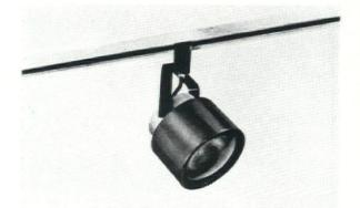
direction, and beam position. Lengths of extruded aluminum form a continuous electrified track, in 4and 8-foot modular lengths in straight runs, corners, squares, tees, or crossovers. Track sections, 15/8-inches wide and 15/16 inches deep, can be mounted recessed, pendant, on spacers, or flush.
