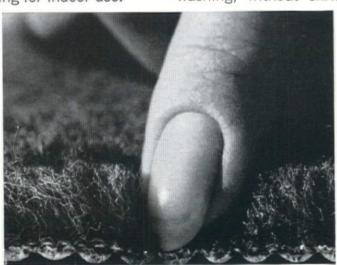
shows no stains with the least care as compared to other carpets, and it lasts and lasts, even after 10,000 abrasion cycles. Comparable acrylic carpet was worn to the backing after 7,600 cycles.
