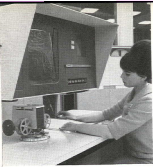
Ampex Corp.'s Videofile (above) records documents on 2-inch-wide video tape—one reel holding 250,000 letter-sized papers. Entries are located and viewed on TV screen, or reproduced full size in minutes. Circle No. 149.
