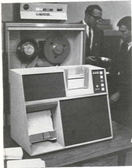
Omnitec Series-300 card readers (above) read the varying punch patterns of different computer brands; re-reads on request. Circle No. 150.
