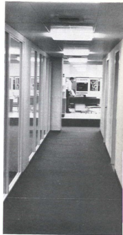
Computer center at Gray Advertising, New York City, was planned and installed by Environment Planning, Inc., design/planning firm specializing in this phase of office design. The computer room is elevated on a raised floor, its base visible at the end of the corridor (above). Key punch room (uppermost left) is on regular floor level. Temperature and humidity are carefully controlled, both recorded continuously and simultaneously on hygrometer (left).
