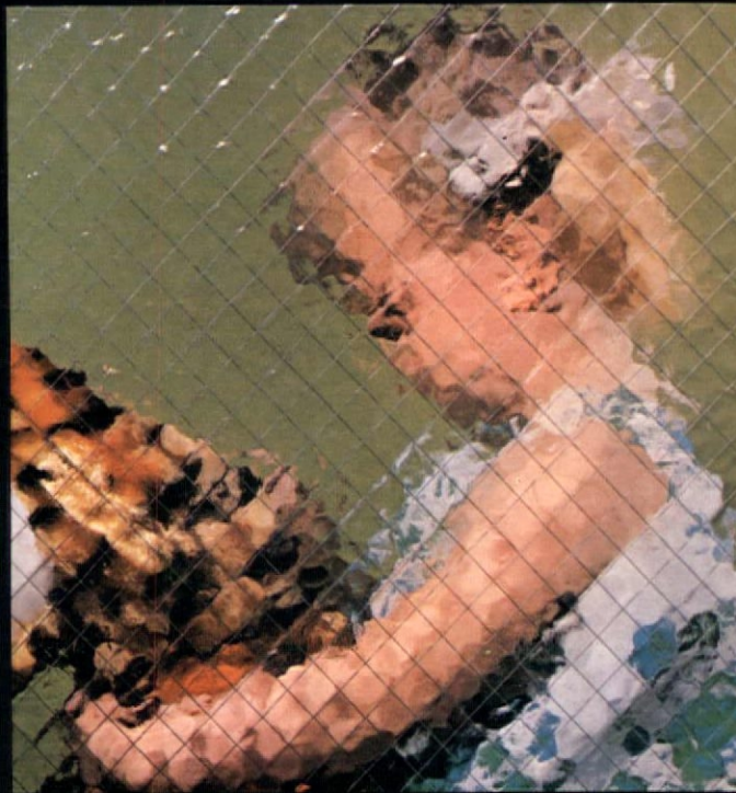
VELVEX NUWELD®. Diamond wire mesh; shallow, slightly wavy pattern on one surface.
