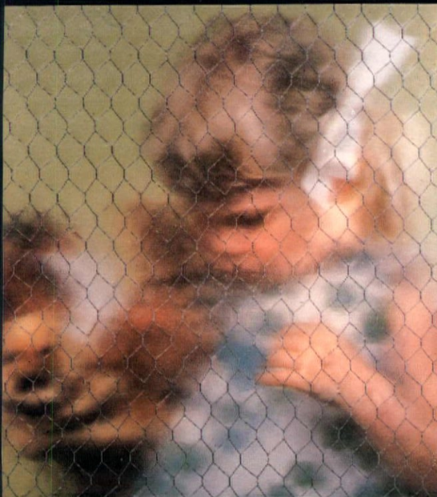
INDUSTREX®. Hexagonal wire mesh; regular pattern of tiny, lens-shaped figures on one surface.
