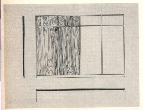
Drawings on this page show the differences between the designer's drawing and the contractor's detailing or shop drawings. At right, the designer submitted this elevation of wall paneling with vertical section at the far left and plan at the bottom. It was translated by the woodworker into the shop drawing above, along with details and sections on the opposite page.
