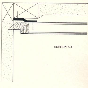
Keyed to the woodworker's drawing on the opposite page, section A-A shows corner of the room where paneling meets plaster; vertical section B-B indicates location of wood grounds and clips for application of paneling; detail C shows shadow line with ¾-inch hardwood recess around all panels. Woodworker's details are reproduced here at 2/3 of original size.
