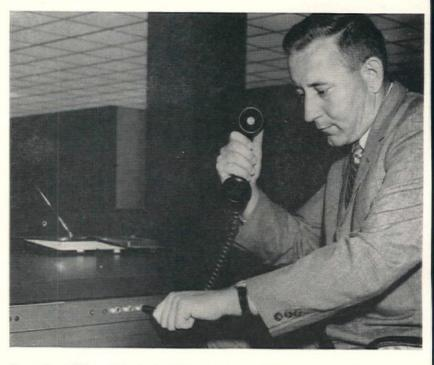
Centralized Edison Voicewriter Televoice transcribing center permits separation of dictator and secretary. Headset plugs into desk system connecting dictator with center located on separate floor.
