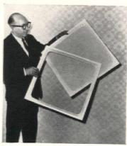
from Dow Chemical is surfaced with 15 mil sheet vin yl which is heated to softening temperature and positioned on the foam frame. The vinyl becomes per manently adhered to the expandable polystyrene and the inner frame is nested with a vinyl outer panel to complete the unit.
