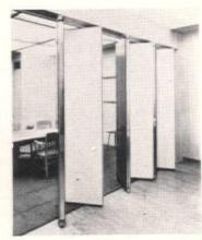
in pairs and operated on an overhead track. Special mechanical seals expand to the ceiling and floor, forming a tight acoustical seal and a rigid wall. The seals are retractable, and no floor track is required. Series 8510 has received a class "E" certification from NSSEA, which covers the range from STC 38 to STC 42. Series 8530 achieved an STC 43 rating.
