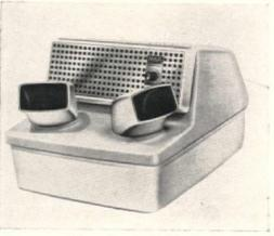
high efficiency filter for individuals requiring dust and pollen-free air. Humidifiers have a 3000 RPM AC brushless motor requiring less than one amp, at 115 volts, 60 cycle. Tank holds one gallon and output is approximately three gallons every 24 hours. A stainless steel spring clip snaps out to release the pump for cleaning. All major parts are made of high impact plastic, eliminating rust.
