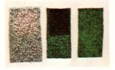
Nylon 100 hours Polypropylene without stabilizers 216 hours Polypropylene with stabilizers Over 2,000 hours Most manufacturers of piece-dyed carpets try for 40 to 60 hours fade resistance. Even stock-dyed carpets strain to reach 200 hours. The special stabilizing chemicals used in the solution-dyed Vectra fiber enables it to resist ultra-violet rays—and permits Ozite to guarantee its carpet to withstand 500 hours of Fadeometer test without discoloration!
