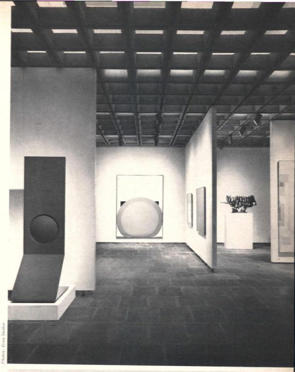
The portable wall system designed by Breuer grew out of the basic design of the building itself, preserving the museum's modular concept. The walls of aluminum honeycombed core wedges fitted between the precast concrete grid ceiling and bluestone floor permit an infinite variety of rectilinear space. The exploded view of the wall system diagrams the floor-to-ceiling Novoply panel wedges and fittings.
