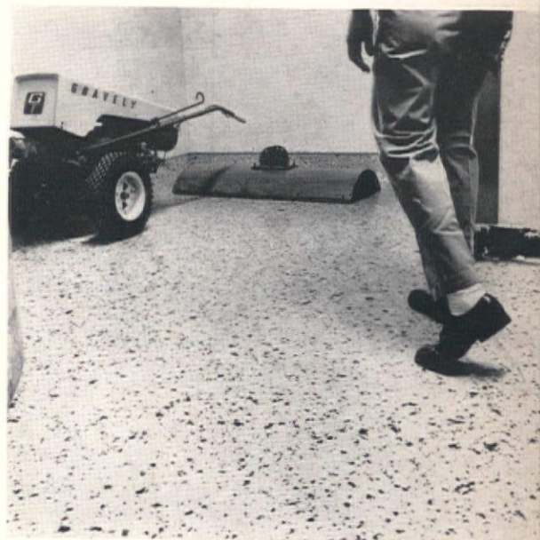
Poraflor Co. demonstrated its product to members of the Hospital Executive Engineers of New Jersey, placing a heavy snowplow, blade down, on a newly installed floor. When plow was removed floor showed neither dents nor scratches. Circle No. 101.
