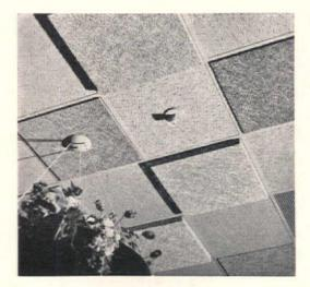
PITTSBURGH CORNING CORP.: Geocoustic unit absorbers were installed on existing ceiling of cafeteria without the need to change lighting or air conditioning ventilators. Each unit is held slightly away from wall or ceiling by integral spacers, thus creating resonant chamber for trapping sound waves. Circle No. 102.
