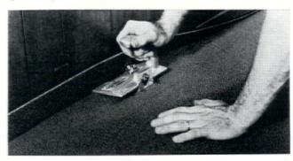
fect-Cut wall trimmer was designed for use with sponge-bonded carpet, it works well on conventional carpeting and allows a more accurate and close cut than that made with a knife. The cutter is crafted of cast aluminum and furnished with six blades.
