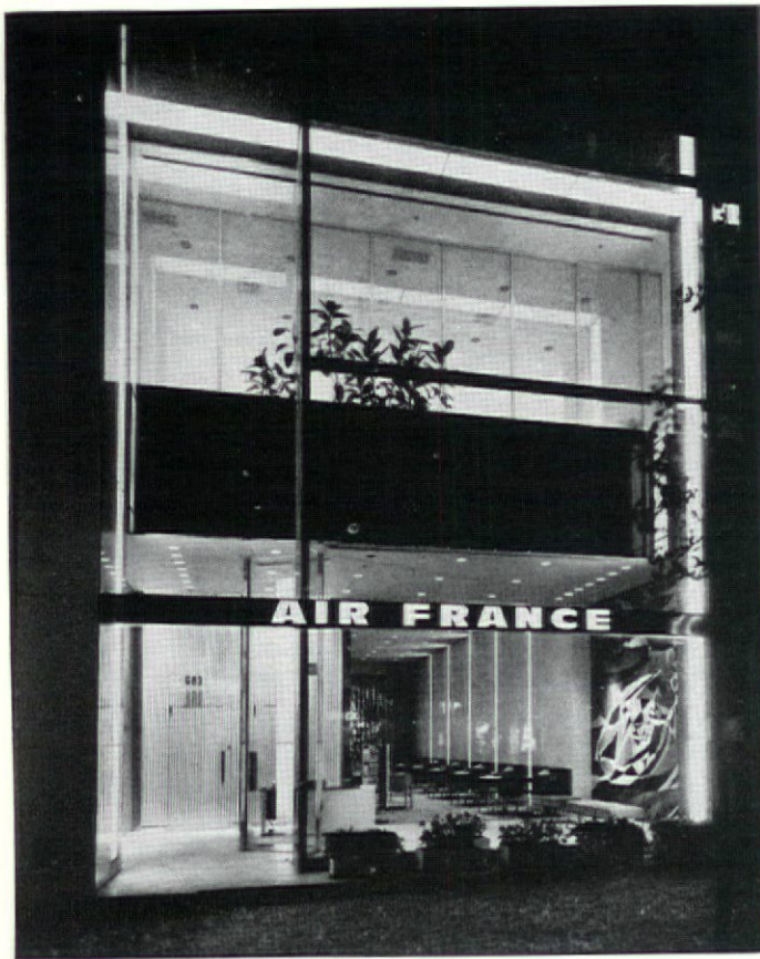
AIR FRANCE ticket office (above) is framed by a continuous band of light to showcase the interior. For Recordak, form and light are combined in a dramatic sculptured ceiling in counterpoint with a three-dimensional floor. Standard fluorescent fixtures are in the deep ceiling wells.
