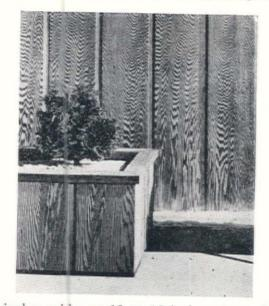
$1\frac{1}{2}$  inches wide, on 12 or 16 inch centers. Long ends are shiplapped for concealed joints. The surface is etched to accent natural graining. The new siding,  $\frac{5}{3}$  inch thick, is available in 4 by 8, 4 by 9, and 4 by 10 foot panels.
