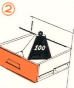
2 NO DEFLECTION, 100 LB. LOADS Grant's 329 Slide will carry loads up to and including 100 lbs./pair, yet remains perfectly horizontal when fully extended.
