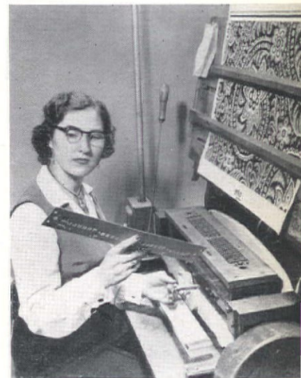
THREE STEPS IN CARPET DESIGN: Left, carpet stylist selects color matches from "quill" boxes containing thousands of hues. Below, artist executes detailed sketch of design on checkpaper, and right, technician uses checkpaper design as guide to punch the cards that are inserted in Jacquard mechanism of Wilton carpet loom. (See cover of this issue.)
