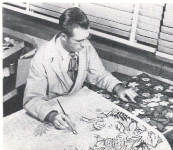
THREE STEPS IN CARPET DESIGN: Left, carpet stylist selects color matches from "quill" boxes containing thousands of hues. Below, artist executes detailed sketch of design on checkpaper, and right, technician uses checkpaper design as guide to punch the cards that are inserted in Jacquard mechanism of Wilton carpet loom. (See cover of this issue.)
