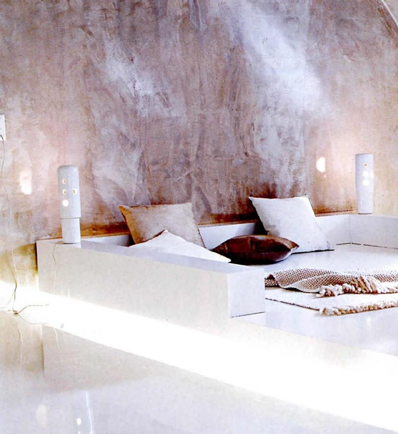
The structural walls are clad in whitewashed OSB. Recessed, dimmable fluorescent lights, reflecting off the glossy floors, illuminate the loft (this page).
