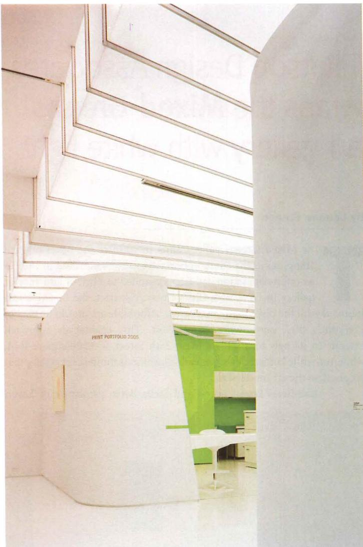
The spacing of the ceiling's flat aluminum support bars varies to establish a strong directional pull from the front to the back of the gallery (above left and right). Sculptural dividers and furnishings are lit by the canopy and exposed fluorescents (below).
