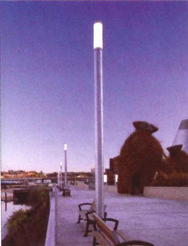
Integrating the SELUX patented MTR refractor technology for glare reduction, MTR Column is a perfect choice for pedestrian and urban area lighting. Choose from three distinct styles in standard heights of 12-, 14- and 16-ft., or in user specified heights. Accommodates up to four T-8 fluorescent lamps, with H.I.D. possible.
