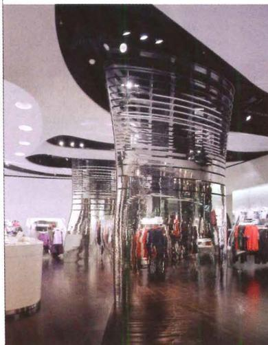
Mirrored chrome, and over 150 hand-bent aluminum strips cover these 15 ft.-high custom column covers. Built for the FILA flagship store in NYC; it won the 2006 NASFM Store of the Year. Just one example of the numerous custom column solutions engineered and fabricated to meet your specifications. View their complete portfolio on the Eventscape web site. "Create without boundaries."
