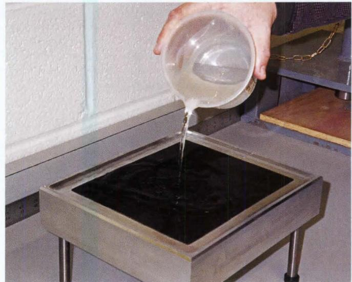
Performing a scrub water exclusion test on a floor box cover.
