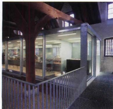
To avoid disturbing archaeological remains in the soil, the new pavilion's foundations are two steel girders that go no deeper than 50 cm. The structure appears to hover above the original floor.
