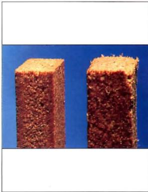
Duraflake MR moisture-resistant particleboard absorbs less moisture & exhibits minimal thickness swell compared to standard particleboard. For interior applications where exposure to high humidity & intermittent contact with water is common. It has a fine surface for laminating & exceptional strength. Applications include bathroom & kitchen cabinets & counters, casework, display fixtures, entryways & other moisture-prone areas. To request information call 1-800-887-0748 ext. 300.
