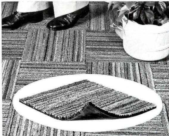
Exceptionally durable in heavy wear areas such as the entrances, lobbies and ramps of airports, theaters, factories and shopping centers. The carpet-like surface is made of heavy-duty tire stock, bonded to a flexible backing, installed with non-flammable adhesive and laid in a beautiful parquet pattern. Tiles are 3/8" thick and 12" x 12" square. (Also golf spike resistant.)
