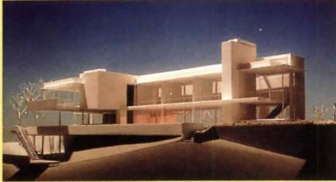
Construction begins this month on a 4,200-sq-ft residence by Edmund Einy on a height overlooking Santa Monica Bay. A movable glass-wall perimeter around a light-gauge steel structure on a 16-sq-ft grid blurs distinctions between outdoors and the open-plan interior. A bermed lawn and an upstairs screen wall provide street-side privacy, but a skylight the length of that side compensates for lost contact with the outdoors. ■
