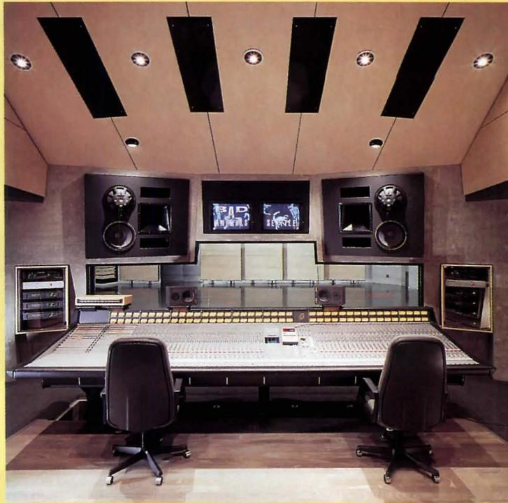
*In the control room, acoustical absorption, reflection, and diffusion devices focus sound symmetrically.*
