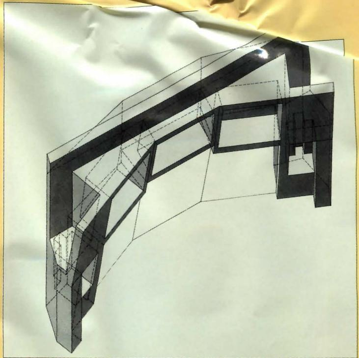
A concrete frame contains both audio and video monitors. Stud walls separate this structure from the recording studio.
