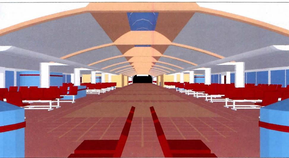
**AutoCAD's 3-D models are complemented by AutoShade's rendering capabilities. This rendering places the viewer at the end of one of the airside terminal's wings and looks toward the center of the building.**
