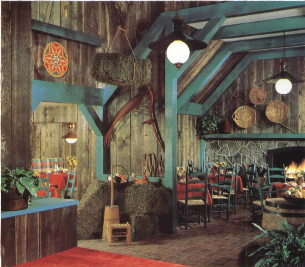
Georgia-Pacific introduces wall paneling with the rustic, mellow look of weatherworn barn board. New Barnplank paneling is a 5/16"–4' x 8' panel with a face veneer of real Ponderosa pine. All natural markings in the veneer, such as knots, splits and worm holes, have been retained.
