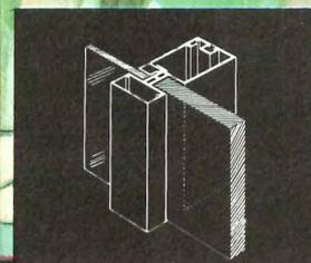
One extrusion can accommodate glass or panels of different thickness.
