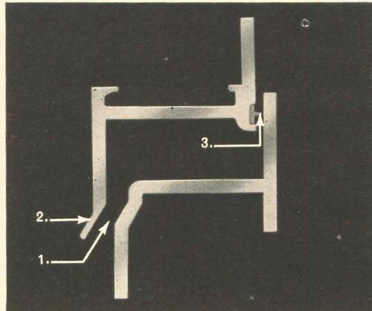
**Triple Weather Guard**—1) Pressure equalization slot, 2) integral drip, and 3) neoprene weatherstrip. The Sealair window offers triple weather protection. Weathering where needed, scientifically designed.
