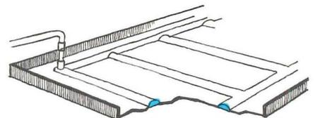
Cross-section of Inland IRC/HP panel shows two layers of heavy-gauge steel brazed together to form water channels across the top surface. 2' x 4' modules fit standard lay-in ceiling grids, simplifying integration with lighting panels and partition systems. Self-contained water channels free designer to create imaginative ceiling effects without expensive plumbing installations.
