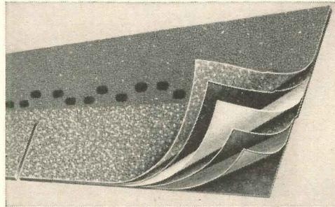
Ruberoid FIRE-GUARD 325-lb. residential shingles feature a built-in, special fiberglass blanket, in addition to other flame-resistant layers. U.L. puts these self-sealing shingles in top Class A rating for fire and wind resistance. Good looks too, in 6 modern colors!
