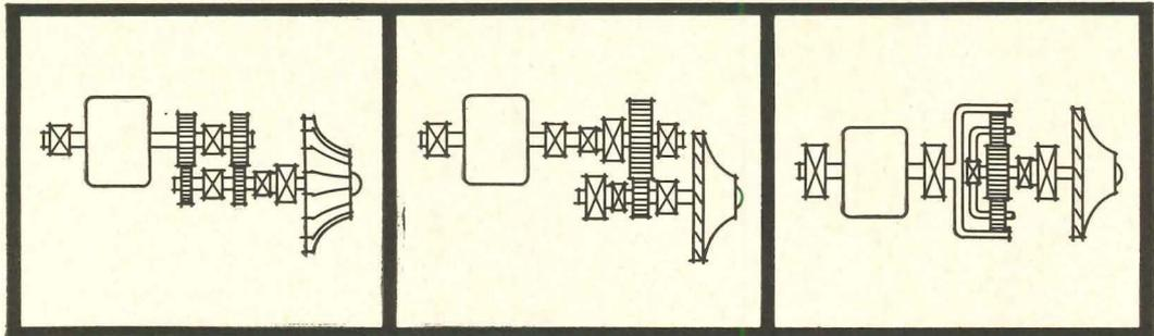
**Make "A"** Gear-drive, including four gears, three bearings, plus a high-load thrust bearing.
