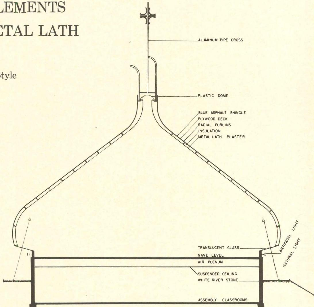
Laminated wood arch ribs and radial purlins form the main structure of St. George Syrian Orthodox church designed by architect John Michael, A.I.A. A metal lath and plaster ceiling was formed to follow the curve of the roof between the exposed arches. Roofing is shingles over plywood deck.
