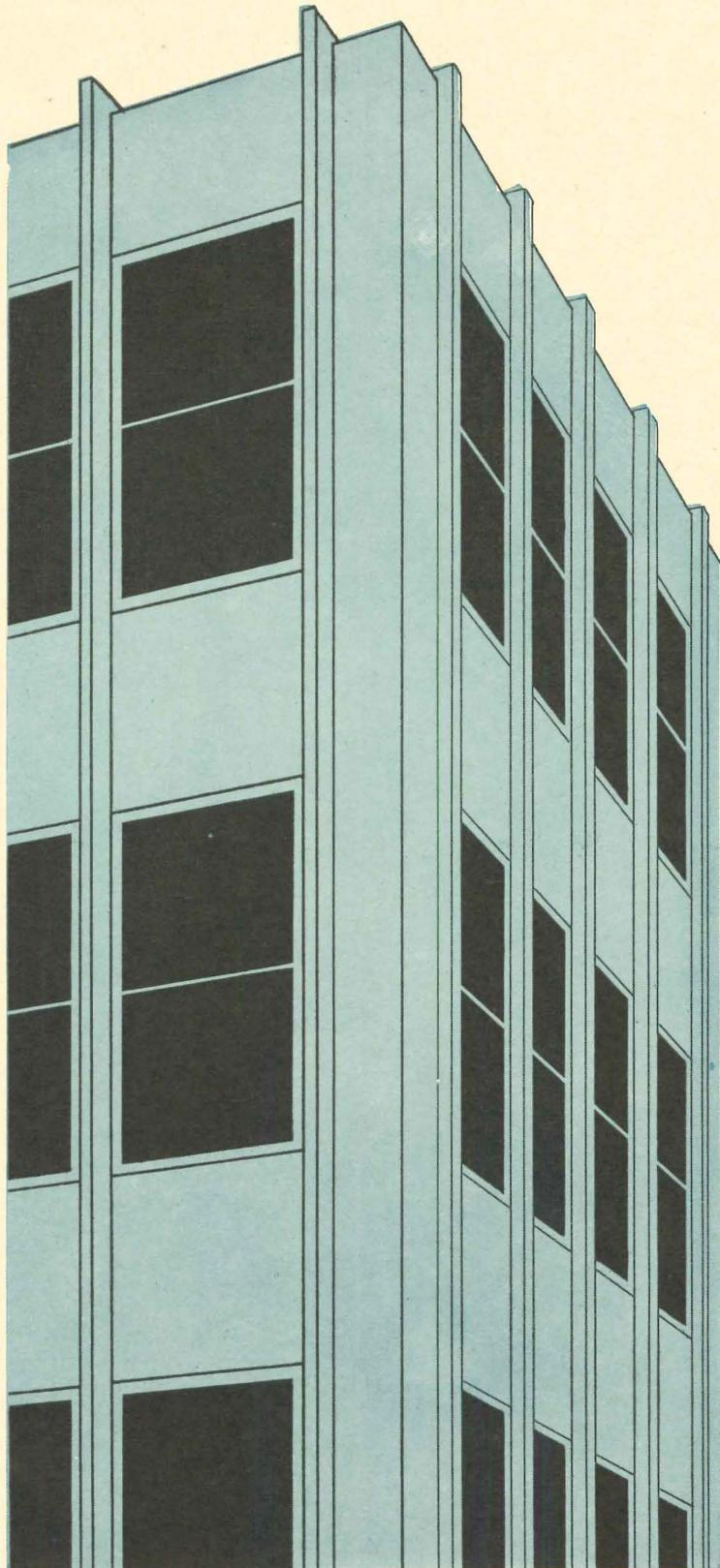
**1. Perfect color match:** That's because finishes of Kynar 500 are liquid . . . can be roller coated on to flat metal stock and post formed . . . the same color finish can be sprayed on to metal parts. You can now color-match mullions, trim and curtain wall.
