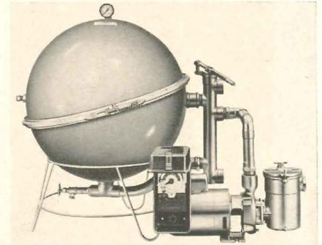
filter is a diatomaceous earth filter which is only 25 ins. in diameter and thus occupies considerably less space than the several sand filters which would be needed to produce a comparable flow rate. A self-cleaning process enables the filter to operate for long periods before backwashing and cleaning is required. The backwashing and cleaning operation is initiated by simply moving a lever. *Culligan, Inc., Northbrook, Ill.*
