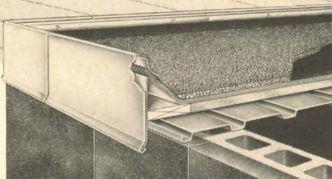
Hickman System prevents water leaks at eaves—stops tar drippings. Note attractive aluminum fascia available in 4 finishes.
