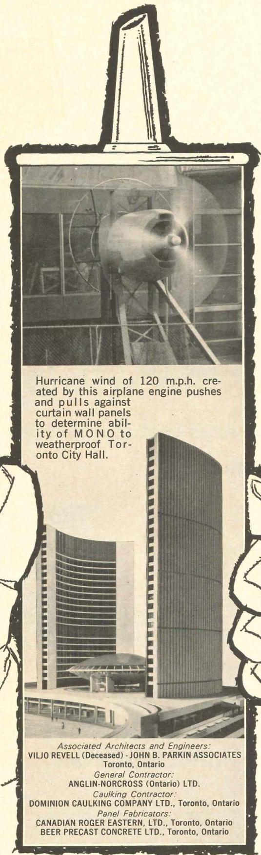
Hurricane wind of 120 m.p.h. created by this airplane engine pushes and pulls against curtain wall panels to determine ability of MONO to weatherproof Toronto City Hall.
