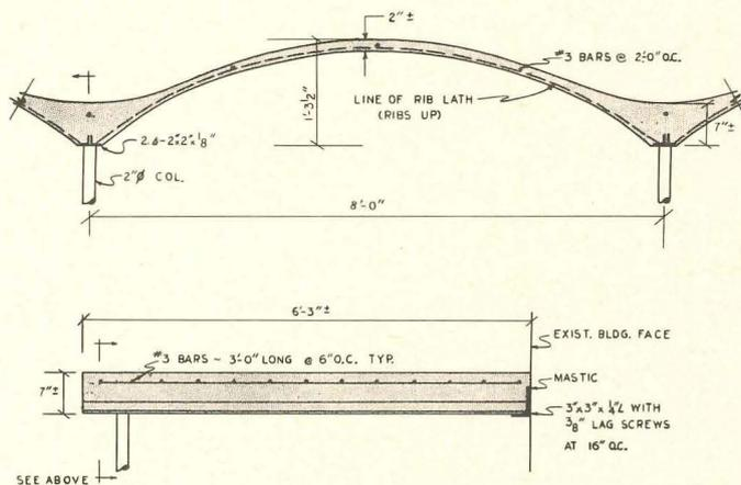
Reinforcement for the 8-ft span was more than adequate.
