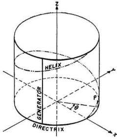
A cylinder is generated by a straight line element (the generator or generatrix) which moves along a plane curve (the directrix) parallel to an axis which is not in the plane of the curve. When the axis makes a right angle with the plane of the curve, the surface is called a right cylinder. For design purposes we can always arrange the cylinder to be right.
