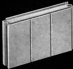
**NEW Fenestra Type "C" Wall Panel** — Smooth flush surface. Factory assembled. For use either horizontally or vertically in walls or partitions. Grained aluminum or galvanized steel. Width 24". Lengths to 14'. Depth 3".
