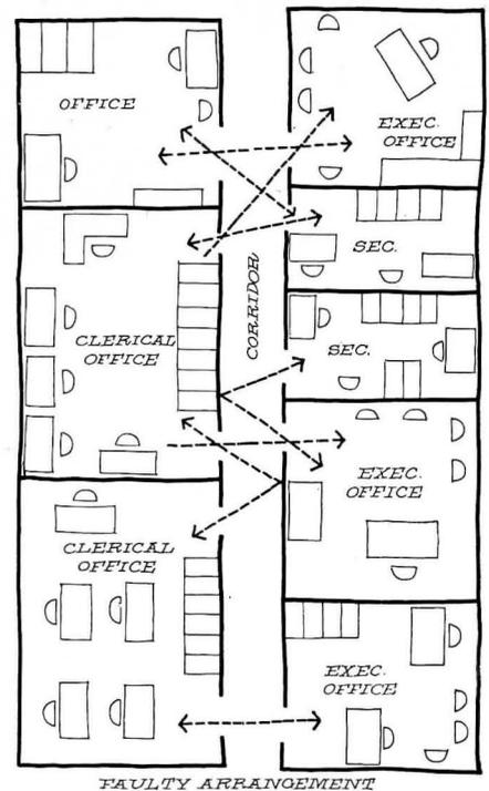
Fig. 2. A faulty arrangement of offices along a corridor. The presence of many doors at one point makes noise transmission likely, and it also causes traffic concentration in these areas
