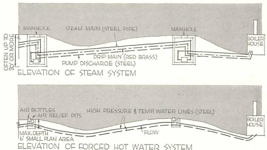
Hot water system piping can easily follow the contour of the land—the circulating pump takes care of any changes in elevation. With steam systems, pipe lines must be pitched down in the direction of flow to drain properly, and must be dripped at all low points. Red brass is usually used for drip mains to cut down on the amount of erosion. Red brass for the large steam main would be too expensive
