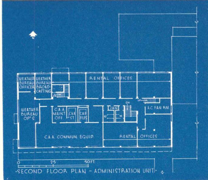
Second floor of administration unit (plan at left) contains weather bureau, CAA offices, rental space. As in all air terminals, official spaces here and in control tower floors (controller offices, radar room, control cab) contain much special equipment required by regulations, with provision for more and different future equipment
