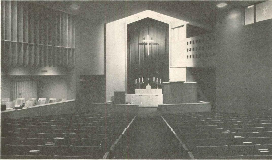
*Non-parallel enclosing surfaces produce desirable acoustic properties in sanctuary. Only acoustic treatment is absorbent plaster in center ceiling panel. Although choir (below) is at one side, no noticeable variation in intensity or quality of sound has been reported*
